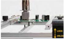
Supports P.W.B. from underneath to minimize its warping.
